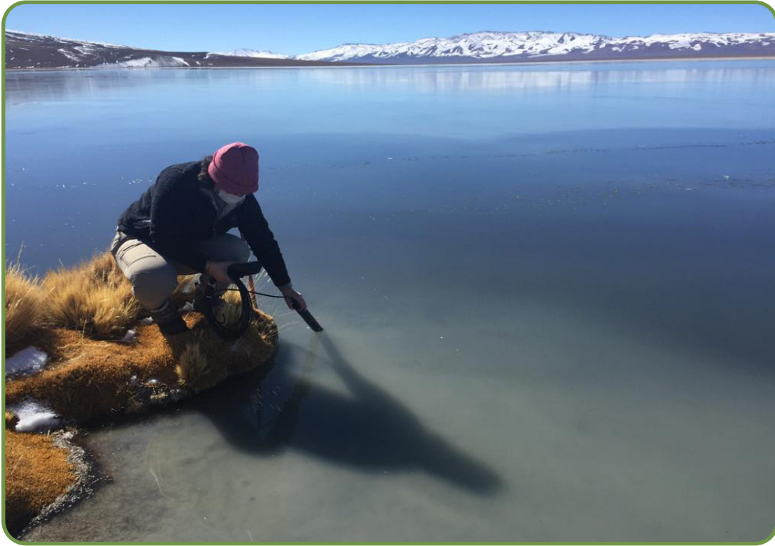
Photograph: Lagoon monitoring with multiparameter probe.
