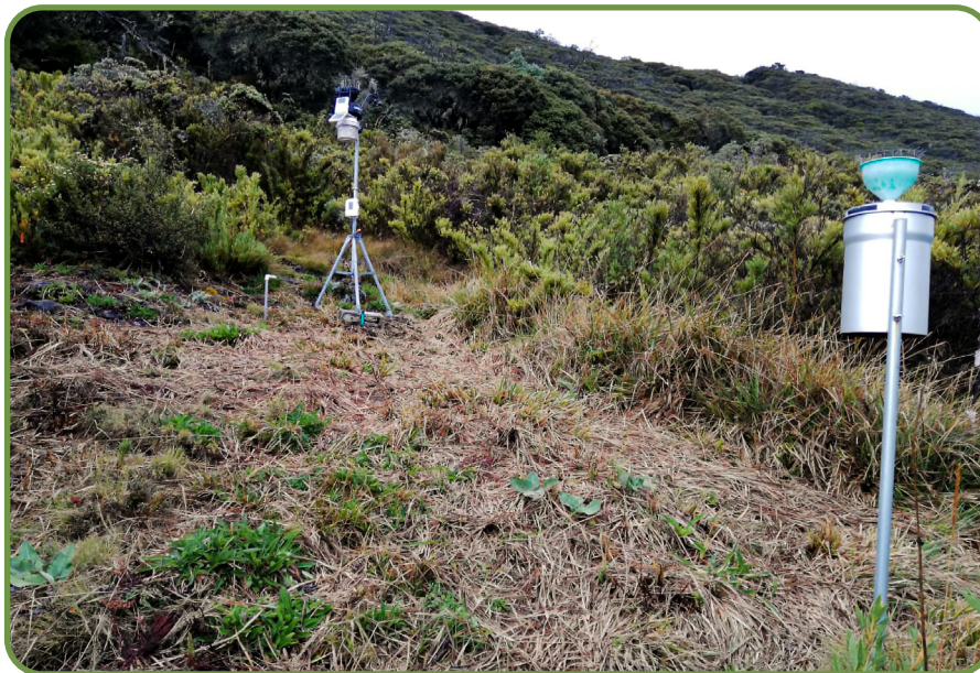
Photograph: Automatic weather station (in the background) and the rainwater sample collector for isotopic analysis (in the front).
