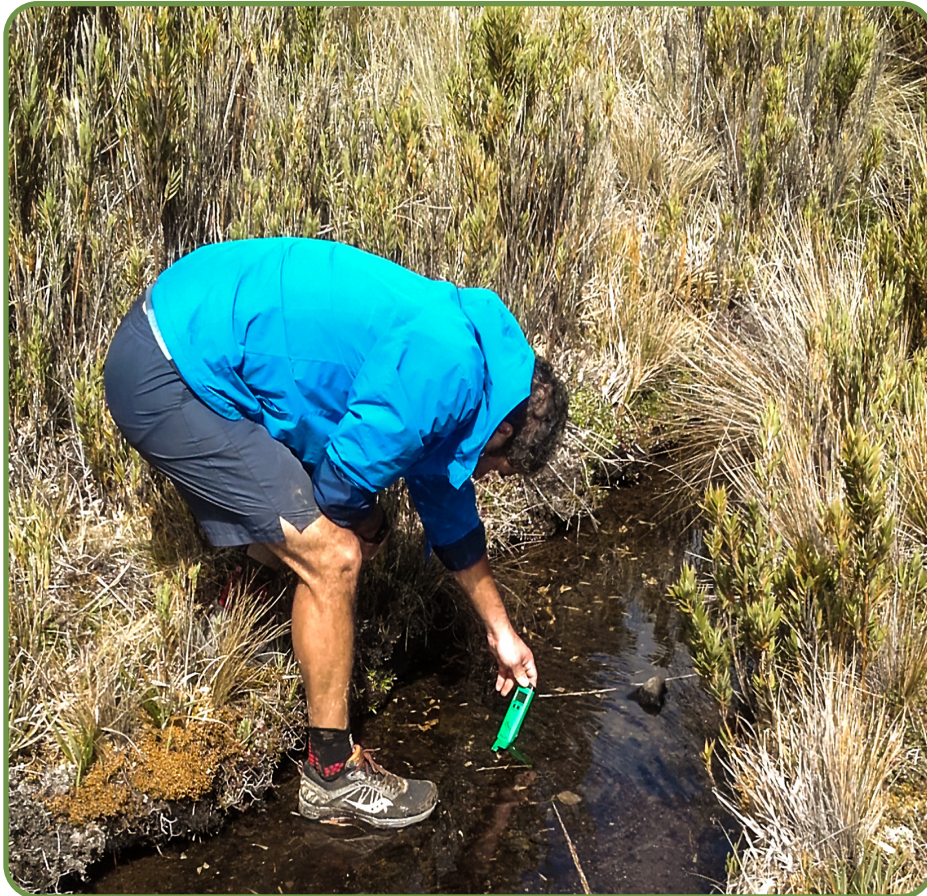
Photograph: Measurement of pH, temperature and electrical conductivity in the surface water systems of Páramo de Chirripó.
